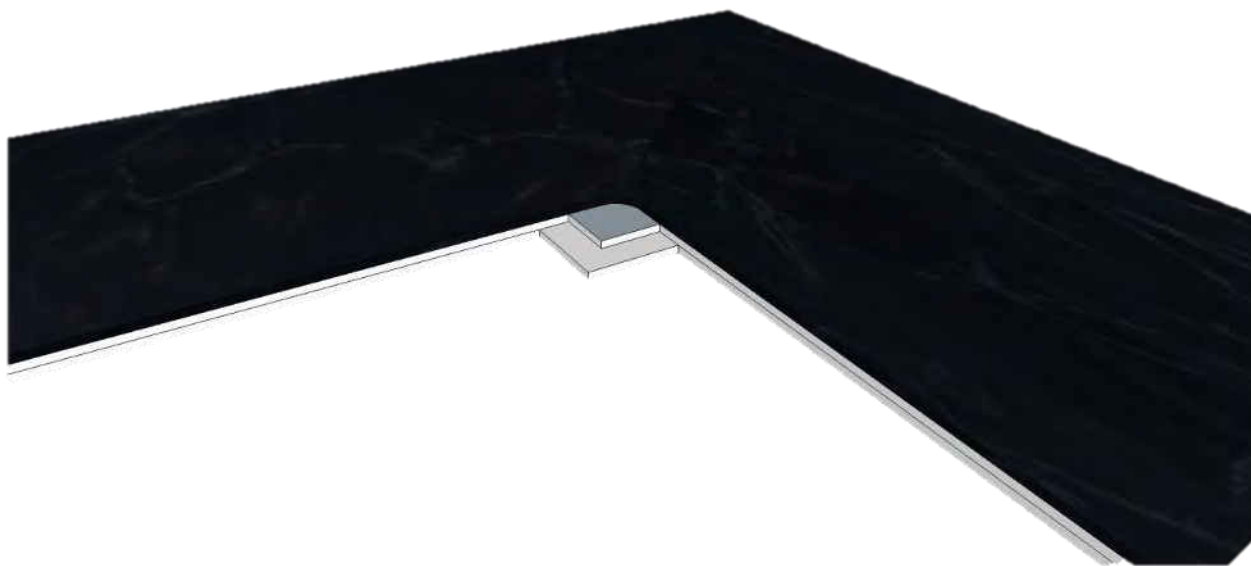
Figure 14. Veined miter joint topside utilizing the “Interlocking Corner Block Method”
