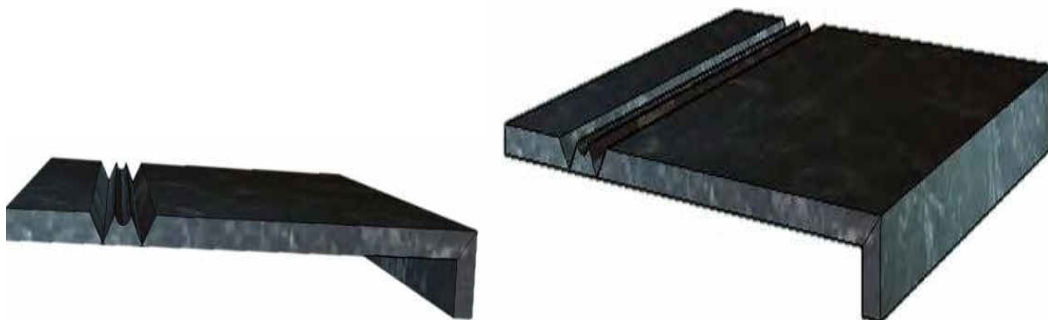
Figure 21. V-Groove edge before gluing and folding
