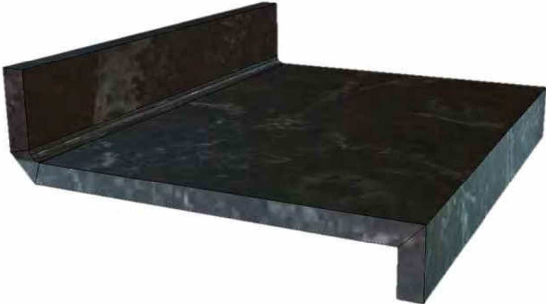
Figure 20. V-groove technique folded together
