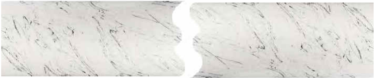
Figure 5. Serpentine deck seam, cut mirrored joint shape
